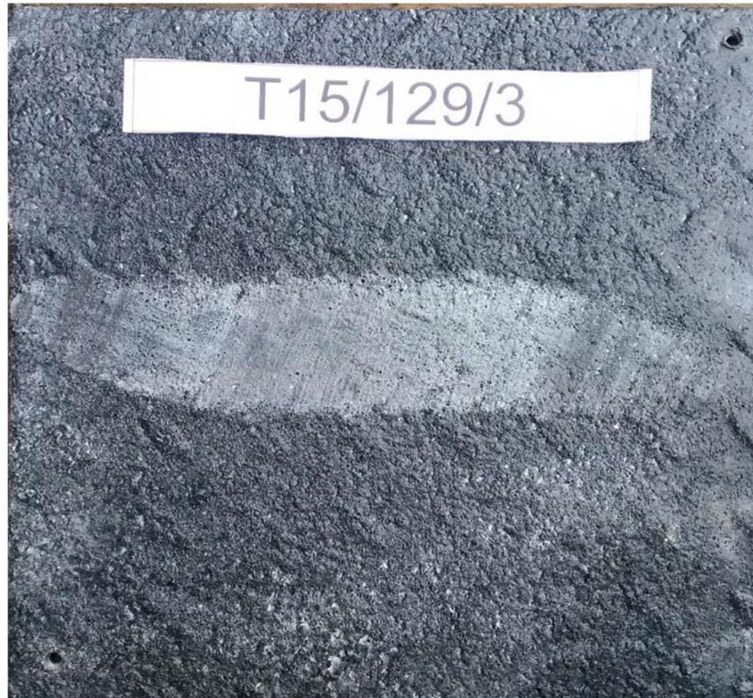
After 500 wheel passes at 35°C
